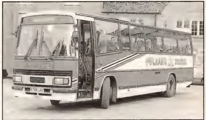
The three piece screen and twin leaf doors of a Paramount 3200 Express bodied Leyland Tiger at the Bourton terminal of the main Cheltenham service.
